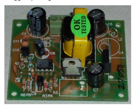
Solar Charge controller with BUCK and BOOST function using advanced two step PWM technology
